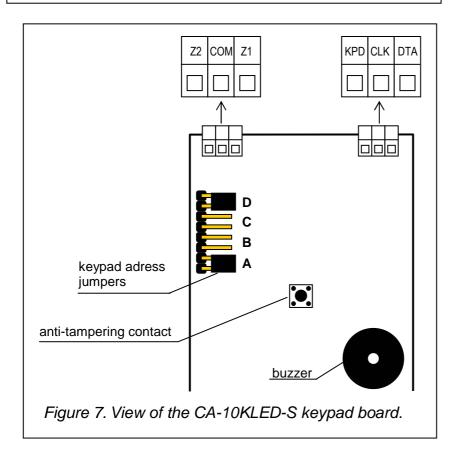
The keypad anti-tampering contact has no connection with the system anti-tampering circuit. Its state is defined by the control panel, based on the data received from the keypad. When the control panel is in the service mode, the anti-tampering contact is not controlled.
