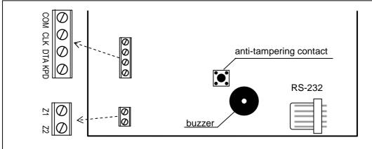
Figure 5. View of the CA-10KLCD-L keypad board. The CA-10 KLCD-S board only differs in its outside dimension.
