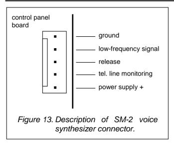
Where the function of alarm messaging with voice announcements is used, a voice synthesizer must be connected to the control panel.
