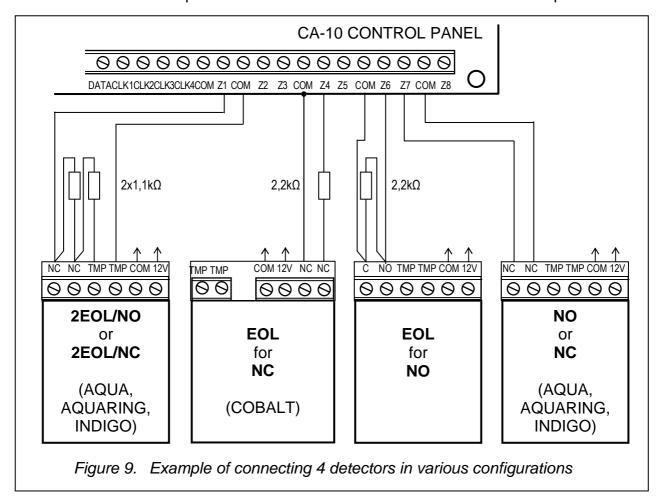
Figure 9 shows how the detectors should be connected to zones working in various configurations. Separation of the detector power supply ground and the line ground makes it possible to eliminate the harmful effect of wiring resistance. Assuming that the wire is rather short, and only one detector is connected to it, the installation can be simplified by using one wire for the power supply ground (GND) and the signaling ground (COM).
