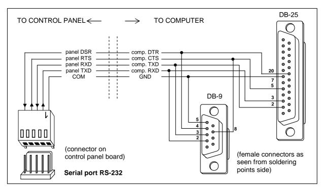
Fig.15. Connection of computer to the control panel serial port.
