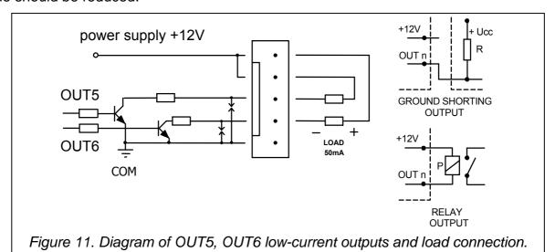
Where signaling devices with their own internal battery are employed, the OUT4 output can be used to power the signaling devices, and the triggering signals can be provided by the OUT5 and/or OUT6 low-current outputs.
